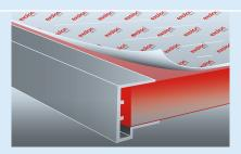
**10** | When sealing sheet ends there is a simple, but very important, rule to follow which keeps condensation to a minimum: seal as tightly as possible at the top (e.g. seal edges with aluminium tape and if necessary affix an aluminium-end profile, possibly with seal), and as tight as necessary at the bottom (e.g. seal with anti dust filter tape and affix an aluminium end profile). Any water penetrating the end-closure section from outside must be allowed to flow off (without pooling).
