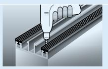
**3** | Install the base section of the glazing bar to the rafter. The edge section seals the sheets at the sides of the roof.
