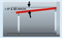
2 | We recommend a roof pitch of at least 5° (≙90 mm/m) to allow rainwater to flow off better. This has the benefits of maintaining seal integrity and the sheets are naturally cleaned by the rain.
