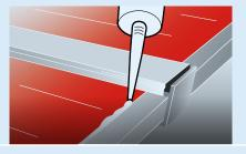
**14** | Seal the upper sealing strip of the end-closure section with silicone rubber that is compatible with Exolon<sup>®</sup> and smoothen it out so that no water can enter.
