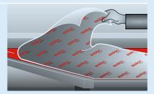
**13** | Finally, remove the masking film from the Exolon<sup>®</sup> multi UV sheets. It should not be exposed to weathering for more than 24 hours.
