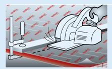
6 | Marking should be done with a soft crayon on the masking film, which should be left on the sheet during machining and until the sheet has been installed. For cutting, use conventional circular saws with unset, multi-tooth carbide-tipped blades. Always work with a stop.
