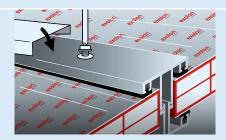
**12** | Peel back the masking film and fasten the upper sections of the glazing bars using the recommended screws with washers. Depending on the glazing system, a cover section is then clipped on.
