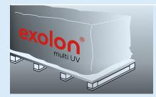
1 | The sheets should be stored flat and indoors, wherever possible. If stored outside, cover the Exolon® multi UV sheets with white polyethylene (PE) sheeting. The chosen supporting structure must be nonwarping. Laminated timber beams or metal supporting structures with longitudinal rafters, on which the glazing bars are mounted, are the ideal choice.
