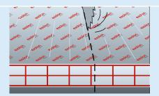
8 | If the sheet width of Exolon® multi UV sheets has to be reduced, please cut as close as possible to the next web to ensure the best clamping action of the glazing bar.
