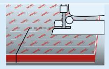
$\label{eq:stars} \begin{array}{l} \textbf{9} \ | \ Corner \ cutouts \ are \ often \ required \\ (e.g. \ for \ pipes, \ ventilation \ etc.). \ Use \ a \\ jig \ saw \ without \ pendulum \ action. \\ Drilling \ can \ be \ performed \ with \ twist \\ drills \ (point \ angle \ \phi \ 110^\circ - 130^\circ), \ conical \ or \ step \ drills. \end{array}$
