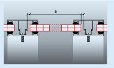
4 | The clear width or sheet width (B) of Exolon® multi UV sheets is calculated from the rafter spacing, the dimensions of the chosen glazing bars and the required allowance for expansion (3 mm/m for polycarbonate).
