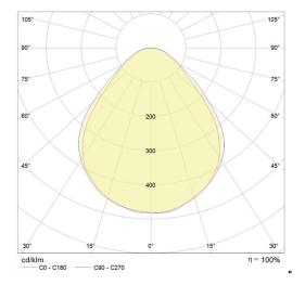
The graph shows how the lenses control the light distribution to allow for efficient de-glaring.
